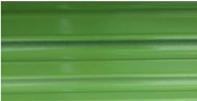
Painting in the Rain, Snow, Fog, etc. (note rain drops in finish)
